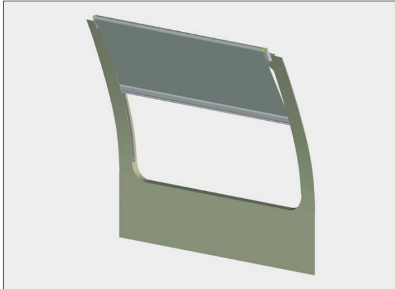
Side panel module with integrated clamp blind DO DB (DB AG double-decker carriage).
