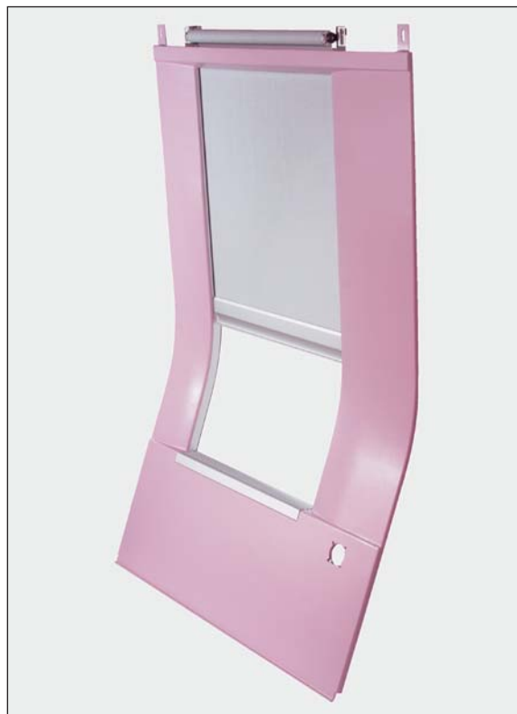
Side panel module with integrated clamp blind DO M6 (Belgian Railways double-decker carriage) (complete aluminium frame with blind screwed onto wall panel from rear. Plug-in ventilation grille).
